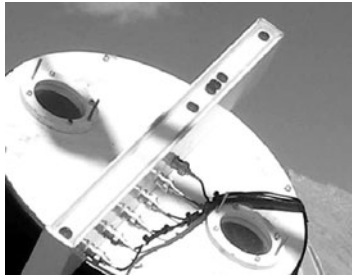
Fig. 4.6 SHABAR uses six photo-diodes attached to a single aluminum I-Beam providing a maximum baseline of 46.87 cm, which was mounted over the telescope with the Solar Differential Image Motion Monitor (SDIMM). The position of the individual sensors in the array are placed at a different locations, which act as a miniature telescopes with 7^\circ field-of-view (FOV). They are separated by 15 non-redundant baselines. The cross-correlations of the measurements over several possible detector separations can be inverted to estimate r_0 as a function of height. This instrument was procured from National Solar Observatory (NSO), USA and installed at the Indian Astronomical Observatory, Hanle (courtesy: S. P. Bagare)
