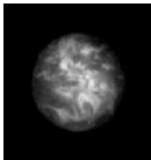
Fig. 7.17 Simulated image of an Earth-like Planet at the focus of a 100 km hypertelescope (courtesy: A. Labeyrie). An image of the Earth picture was convolved with the spread function from 150 point apertures, arrayed in three circles; it was multiplied by the hypertelescope envelope, i.e. the spread function of the sub-pupils as well, and then pushed somewhat the contrast to attenuate the diffractive halo
